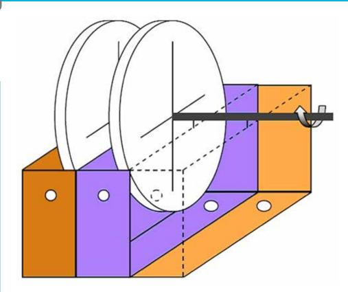
**The system** consists of rotating discs that are partly submerged in either the liquid manure or the receiving sulphur-acid solution.
