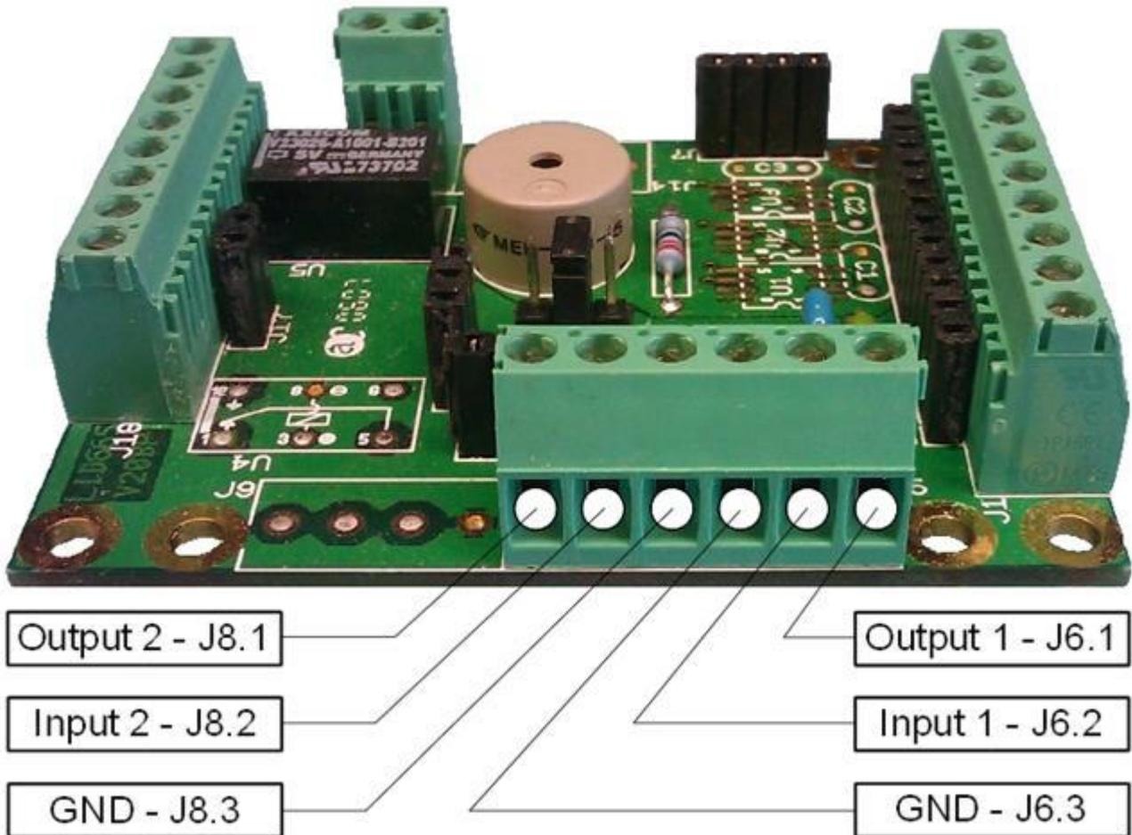
**NOTE:** Use pull-up or pull-down resistors for the sensors (depending on the sensor type)
