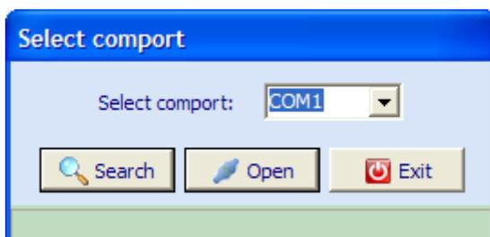
After the software has been installed an icon is created in the START menu. When the program is executed, the comport has to be selected where the program should search for the connected decoder(s). It is also possible to connect using the last used communication type and baudrate by depressing the open button. After depressing the search button the program will try to connect to the reader(s).
