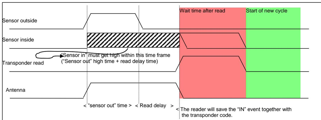
Note: The transponder may be read prior to the inside sensor getting high. In that case, the antenna will be turned off and the reader will continue waiting for the outside sensor to get high.
